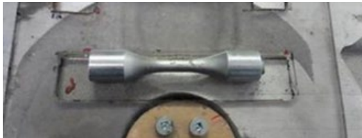
Figure 3a. Example of the template used to ensure the exact placement of tensile and fatigue test blanks within the bulkhead.
